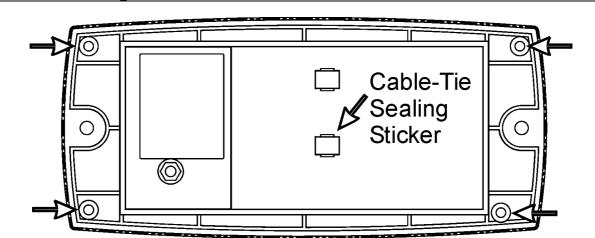
Affix sealing stickers to the rear of the instrument, over one or more screws in the locations indicated.
