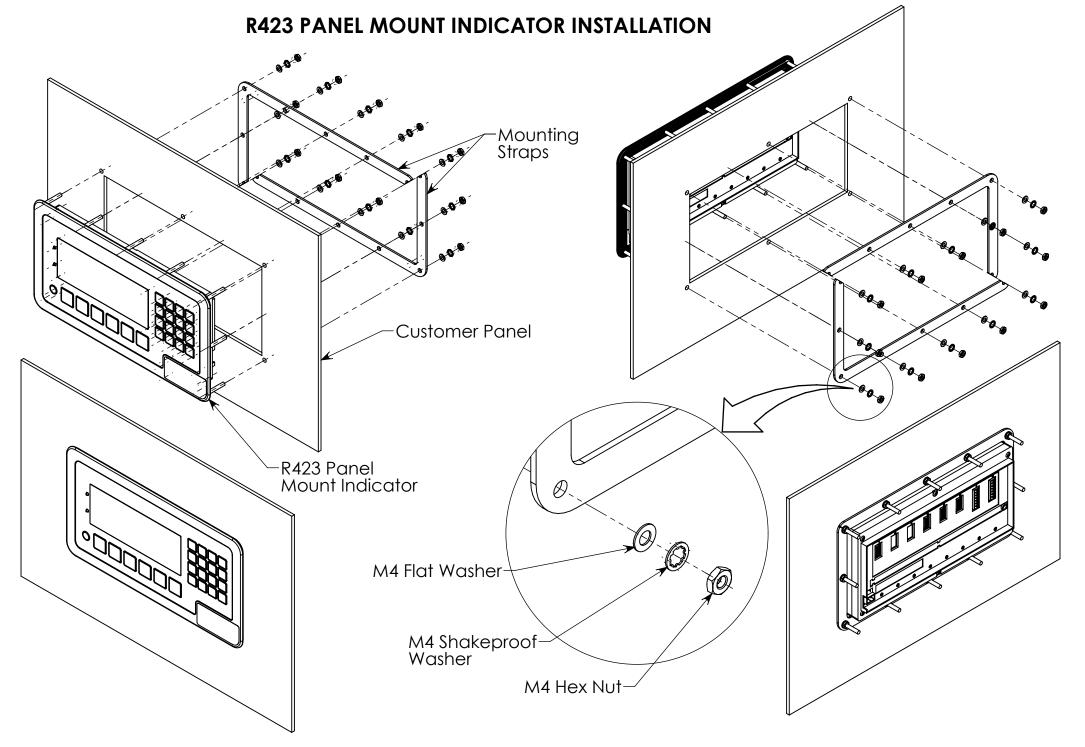
Recommended tightening torque range for the M4 hex nuts: 1.3Nm - 2.8Nm
