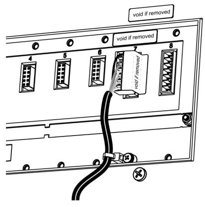
Figure 18: Destructible sticker seal on rear of instrument.
