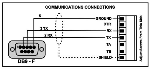
Figure 5: RS-232 - Instrument to PC using COM Port (DB9)
