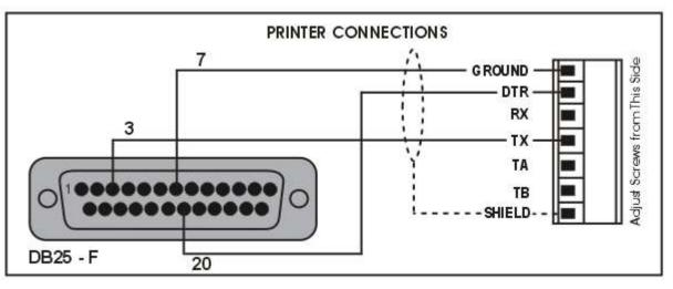
Figure 6: RS-232 – Instrument to Printer (DB25)
