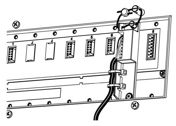
Figure 16: Lead seal on rear of instrument.
