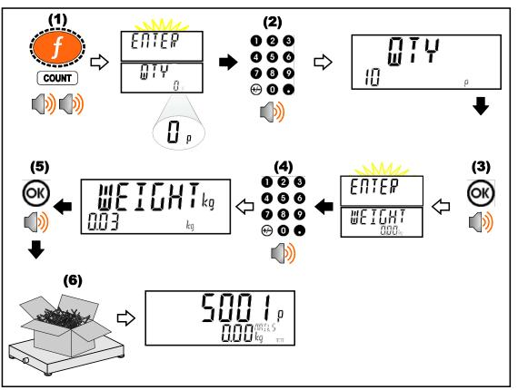
If EDT.WGT is set to OFF then the weight entry step shown above will be skipped and the current weight on the scale will be used. If EDT.CNT is set to
