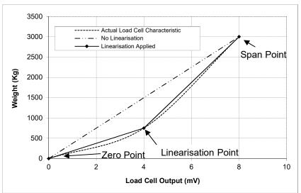
Figure 12: Chart - Non-Linear Characteristic for Load Cell Output
