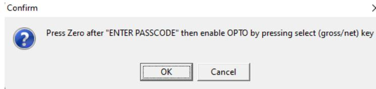
For K342 press Zero Key to skip the activation. Optical Link is enabled by default.
