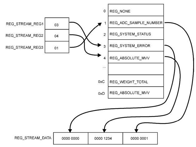
Figure 8: Streaming Registers Example
