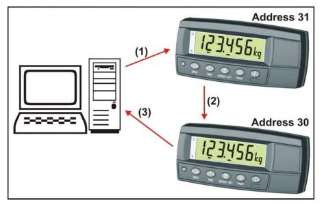
Figure 7: RS-232 Ring Network: Example with Two Instruments
