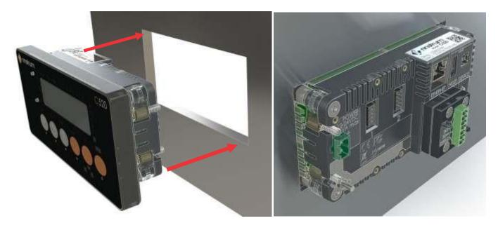
Ensure the clamp screws are backed out so no screw protrudes out the front of the mount brackets, the mount brackets are swung into the body of the C520 and the AC PSU module is not fitted to the indicator.
