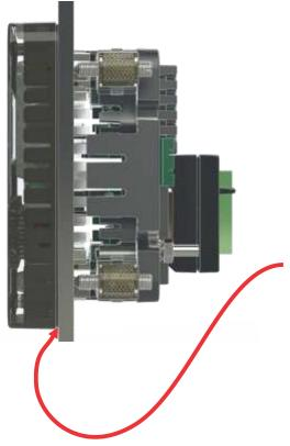
The clamp screws should be tightened until the visible outer edge of the seal on the back of the flange of the instrument is against the front of the panel. This will ensure the sealing ridges on the back of the flange seal are compressed. The effectiveness of the seal will be dependent on the front surface finish, stiffness and flatness of the panel into which the unit is fitted.
