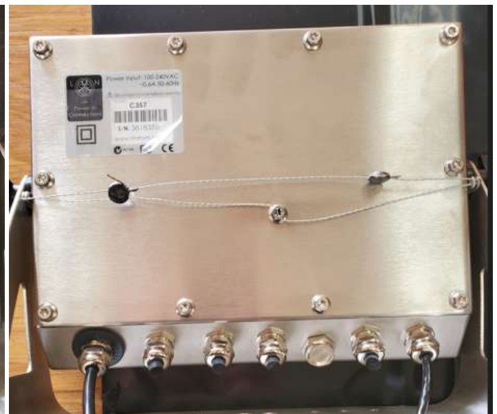
Typical sealing of model C357 / Scellage typique du modèle C357
