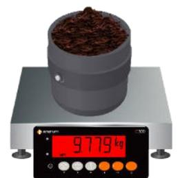
Without Gravity compensation adjustment, this scale would have read 9.779kg
