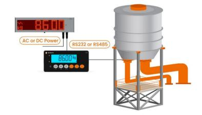
• When the connection is established between the C320 and the remote display, it will mirror the weight shown on the C320 including the unit and decimal points.
