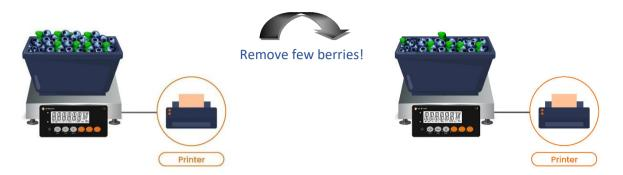
a. When place the filled container on the scale, preset tare weight is automatically reduced from the gross weight and net weight is displaying. But the weight is higher than 1.005 kg (eg 1.009 kg as shown above), display colour will be red and need to remove few berries.
