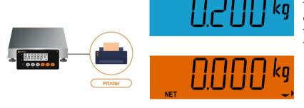
The weight of the empty container should be given as the preset tare. According to this example it is 0.200 kg.
