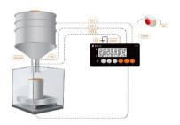
4. Since the FLIGHT is set to 0.3 kg, the FINE will be closed when the bag reaches 24.7kg, and the final weight will settle at 25 kg.
