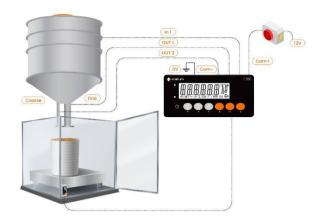
A scale with a C320 instrument fitted is used to control a two-speed filling machine. The final target weight of the bag is 25kg. The filling machine has two separate flow gates for course and fine fill.
