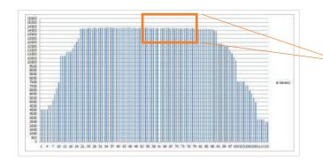
Weighing samples are captured at 100 times per second and then averaged within the offset window.
