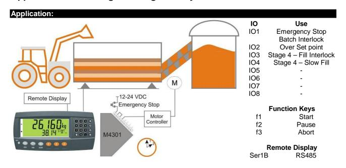
A K411 is used as a controller for a process that does a weigh in, using a front end loader, and weigh out at given time intervals. An example of this would be a bio gas application that uses a weigh in of various materials followed by a weigh out of the mixture on a timed basis into a fermenting silo. The main vessel is filled in this application using a front end loader filling three materials. The mixture in the main vessel is batched out in 1t increments each hour.
