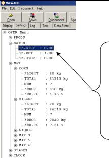
The Batch Timer Details are available through the operator interface on the Recipe key. These can be seen and modified using Viewer by selecting the Session that is OPER.
