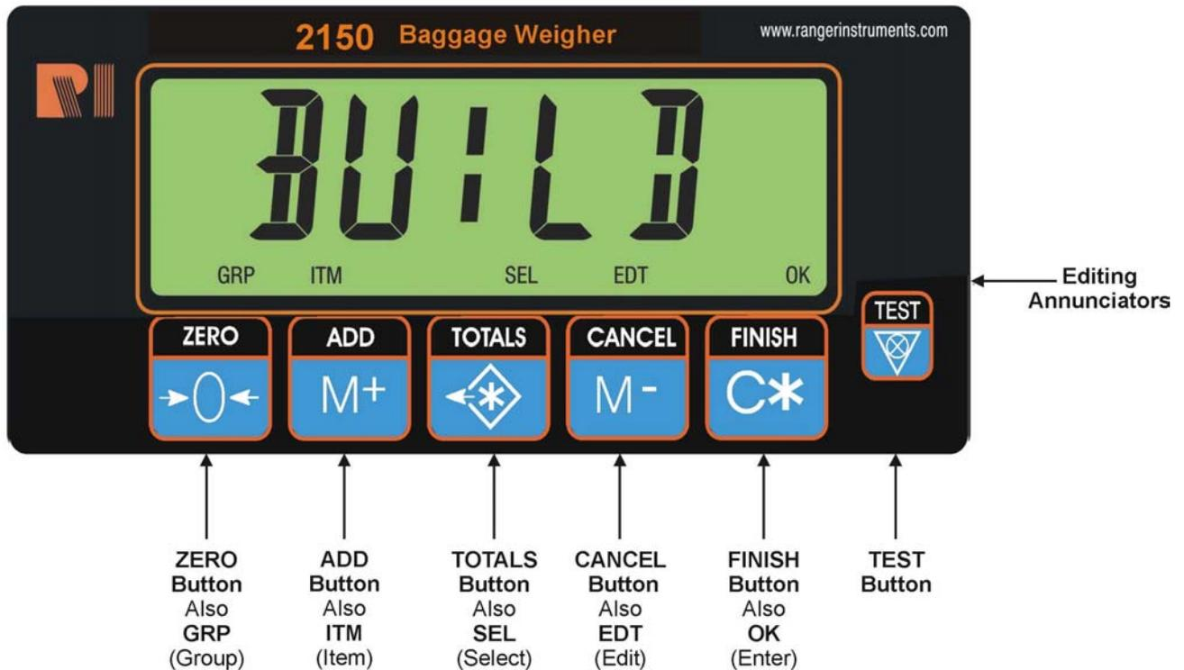
Figure 9: 2150 Setup Display and Controls Illustration
