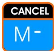
The **<CANCEL>** key is used to cancel the last bag weight. The last bag weight can only be removed once. Subsequent presses of the **<CANCEL>** key result in a long beep. Cancelled bags are printed as negative weights.
