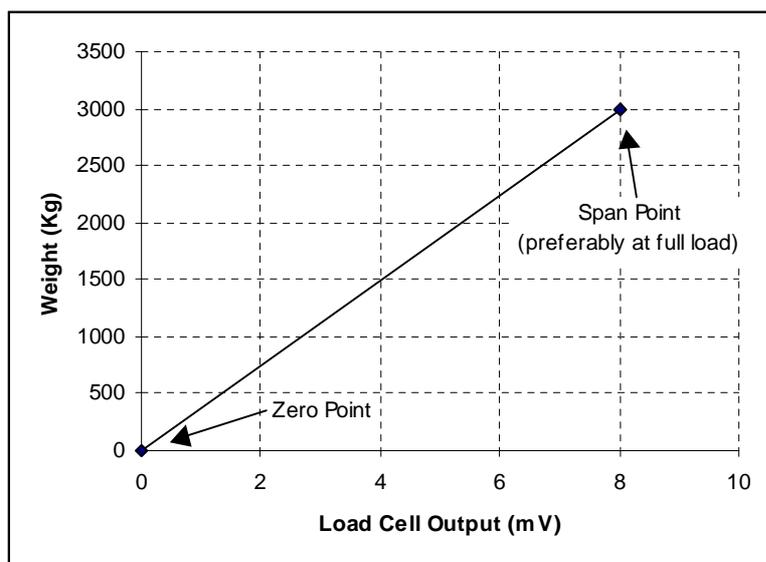
shown here demonstrates how the **5100** uses the zero and span points to interpolate a weight reading from the load cell reading.
