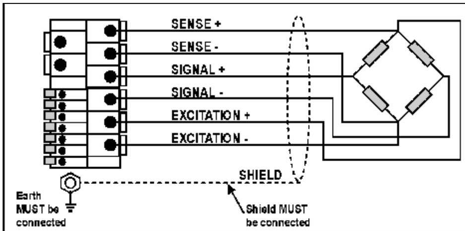
Figure 4: 6-Wire Connections
