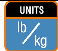
Note: Printing and serial communications will use the units displayed (either kg or lb), but calibration weights and targets, etc., must be entered in the primary display units of the indicator.
