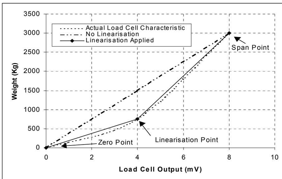
Figure 11: Chart - Non-Linear Characteristic for Load Cell Output
