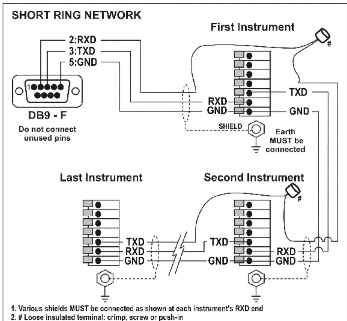
Figure 7: RS-232 Short Cable Runs: Ring Network using COM Port (DB9)
