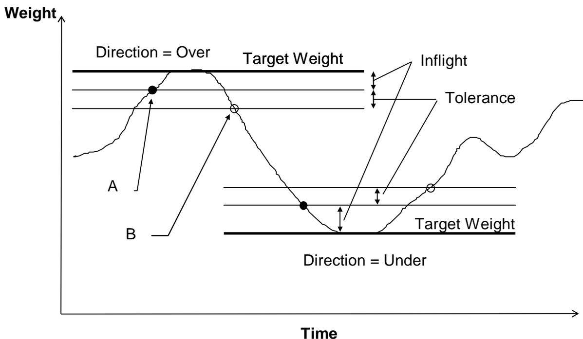
Active Setpoints: Note the difference between Over and Under directions.
