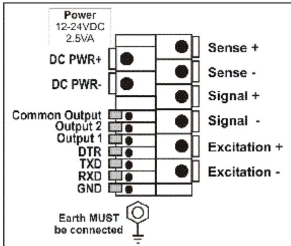
Figure 2: Cable Connections
