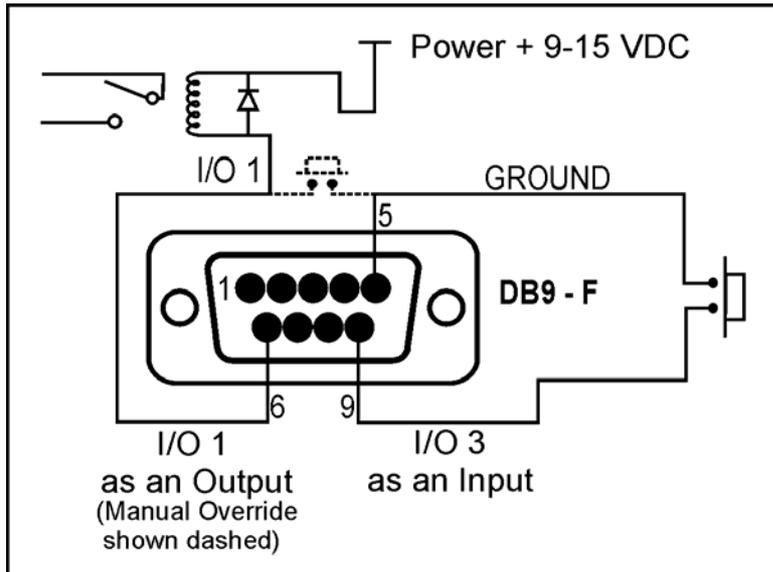
Figure 7: Connection of I/O Pins
