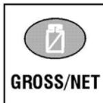
This key toggles the weight display between the Gross weight and the Net weight (provided that a Tare has previously been acquired using the **<TARE>** key).
