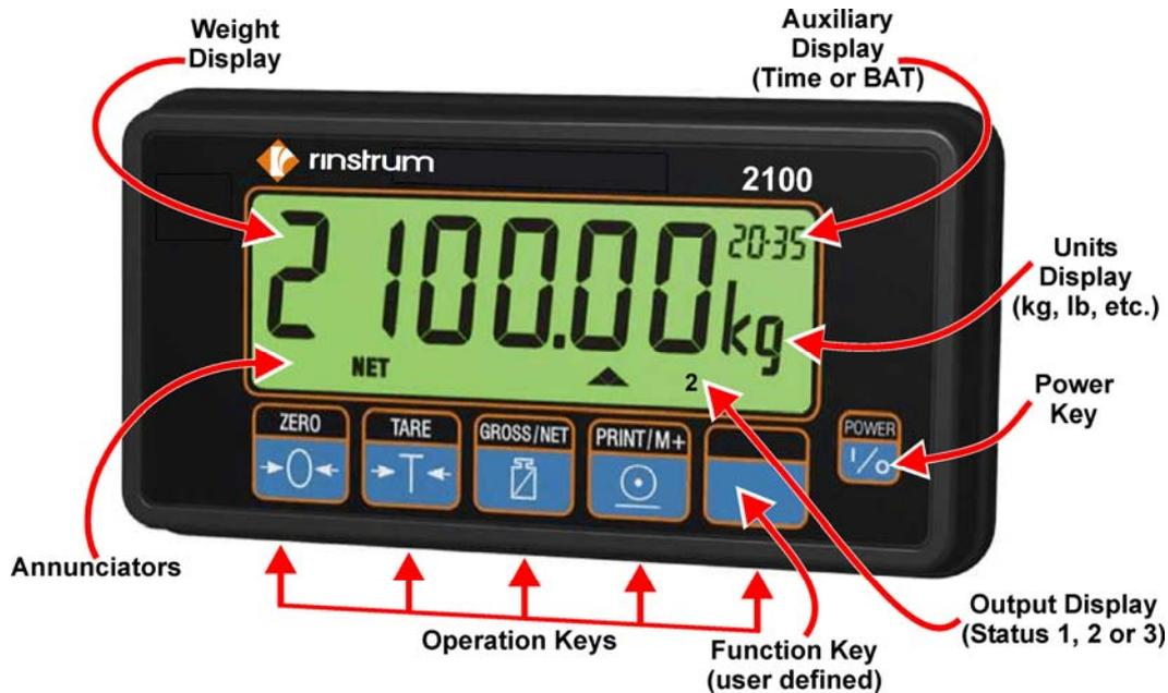
Figure 9: 2100 - Display and Controls Illustration
