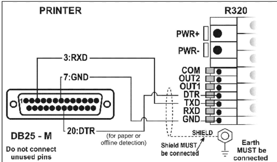
Figure 9: RS-232 – Instrument to Printer (DB25)
