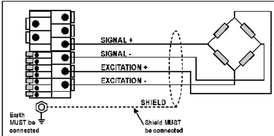
Figure 3: 4-Wire Connections
