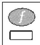
The K35\* firmware allows for the <FUNCTION> key to be configured to a range of special functions. As the K356 firmware allows for setpoints, there is an additional special function available where the key can be used to gain access to the setpoint threshold values.
