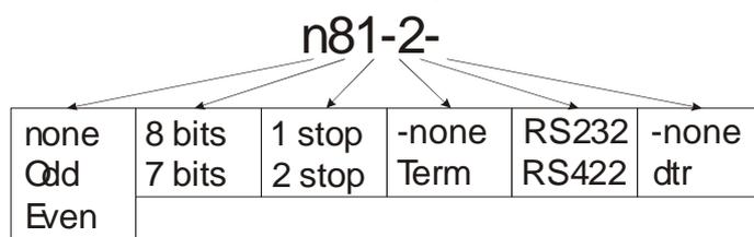
Pressing the OK key will accept the current settings for all options shown. Holding the C key for two seconds will escape from the option entry and cancel all changes to the options.
