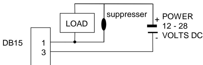
The output stage does not contain a power source and must be powered externally. The external supply should be from 12 to 28 volts DC and the maximum load current must be less than 0.5A .
