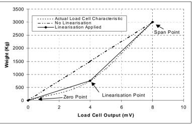
A maximum of five linearisation points can be set independently anywhere in the operating range of the scale. Unused or unwanted points may be also cleared.
