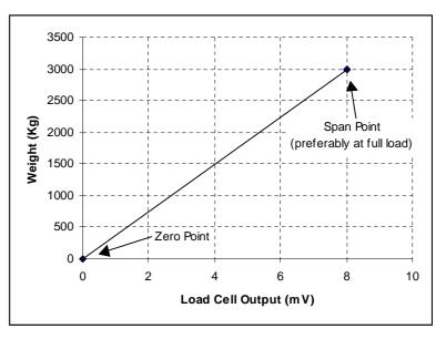
shown here demonstrates how the **5100** uses the zero and span points to interpolate a weight reading from the load cell reading.
