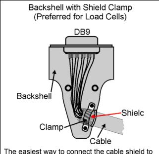
The easiest way to connect the cable shield to the DB9 backshell is to fold the shield wires back over the outside of the cable insulation so the cable clamp of the backshell makes good electrical contact with the shield when installed.
