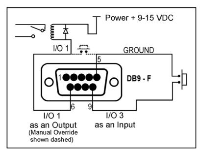
Figure 7: Connection of I/O Pins
