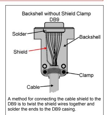
**Figure 3: Cable Shield Connection**
