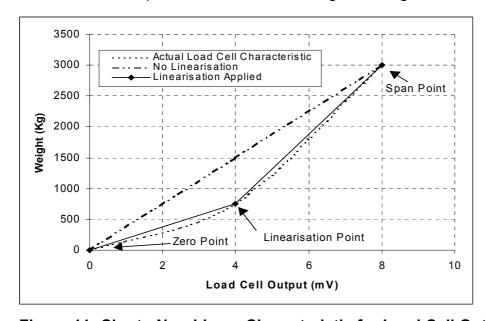
Figure 11: Chart - Non-Linear Characteristic for Load Cell Output
