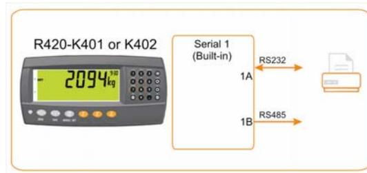
The application requires a **custom print out (Record or Docket)** to be printed from an R400 indicator using a custom print format.
