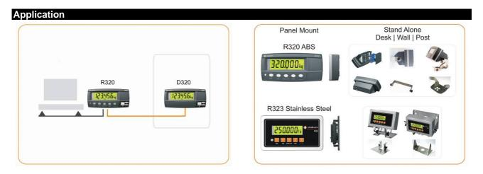
In this example an R320 (or R323) indicator is being controlled by an operator in a control room and a display of the weight reading is required in another area. The D320 remote display mimics the indicator display – using the Master Format.
