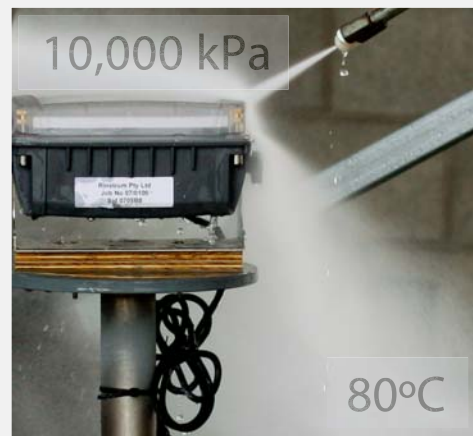
X320 undergoing IP_9K moisture ingress test. High Pressure High temperature water is blasted onto the casing at different angles from 10-15cm away
